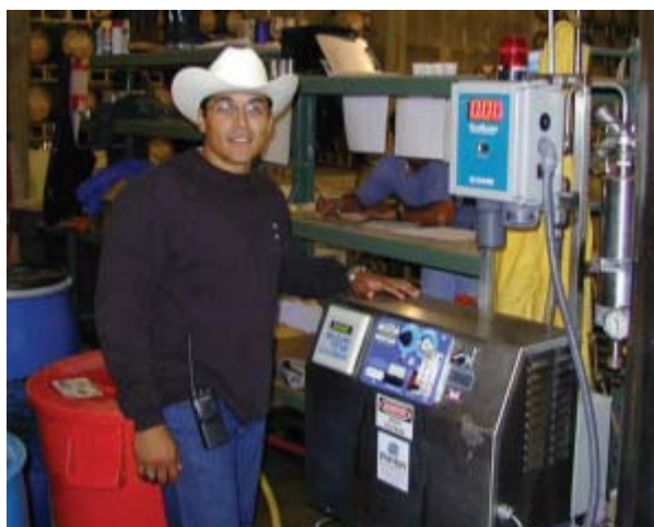
Felipe Martinez, barrel-room foreman at Kendall-Jackson's Oakville facility, standing next to an ozone generator. Note the large ambient ozone display and alarm light on this unit.
